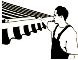
17) With spirit level check if front bar is levelled horizontally.
