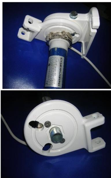
If it is necessary to change drive sides (pin is in the bracket on which you want to install the drive) the pin should be put into the opposite bracket (change bracket axis with pin installation (b) for bracket axis (a)). Both parts will be changed by undoing (de-installation) and securing (installation) of M22 nut with washer.
