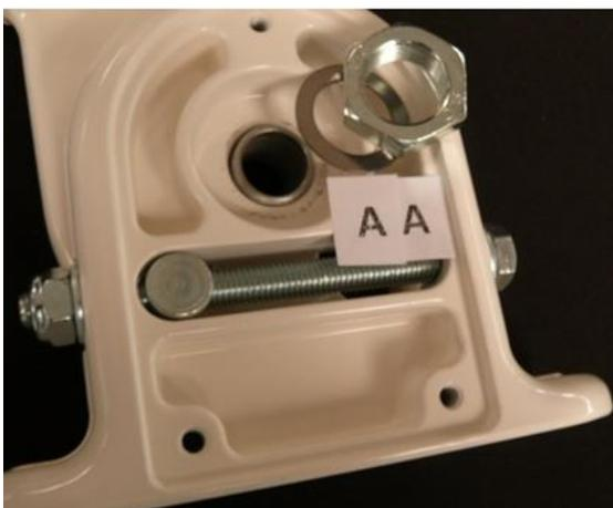
b) With screws fix the motor to movable part with bracket axis and connect again complete bracket.
